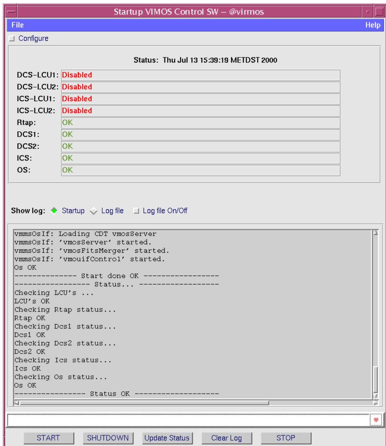
**Figure A.2:** vmmsStart panel. Selecting the “configure” menu (upper left) allows to select the subsystems to be startup or shutdown.
