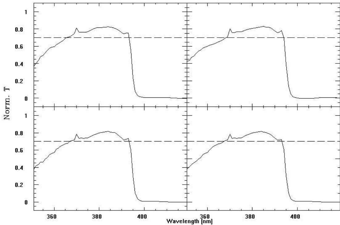
**Figure 19:** U' band filter transmission curves
