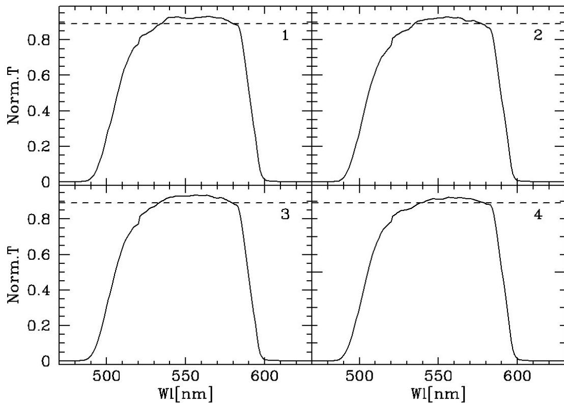
**Figure 21:** V band filter transmission curves
