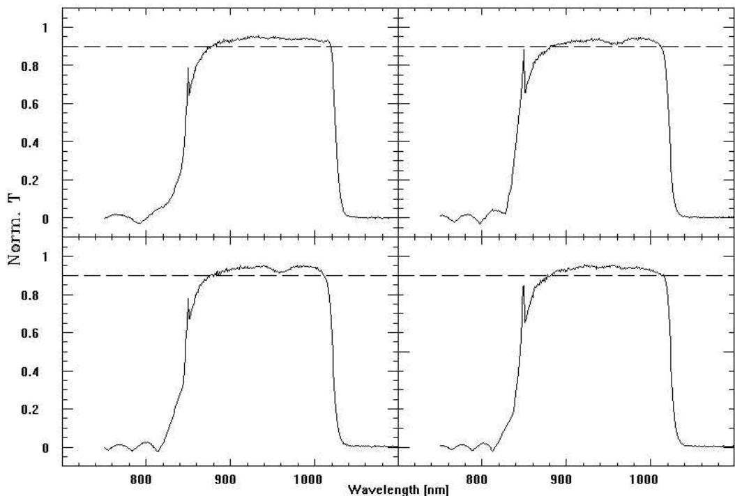
**Figure 24:** z band filter transmission curves
