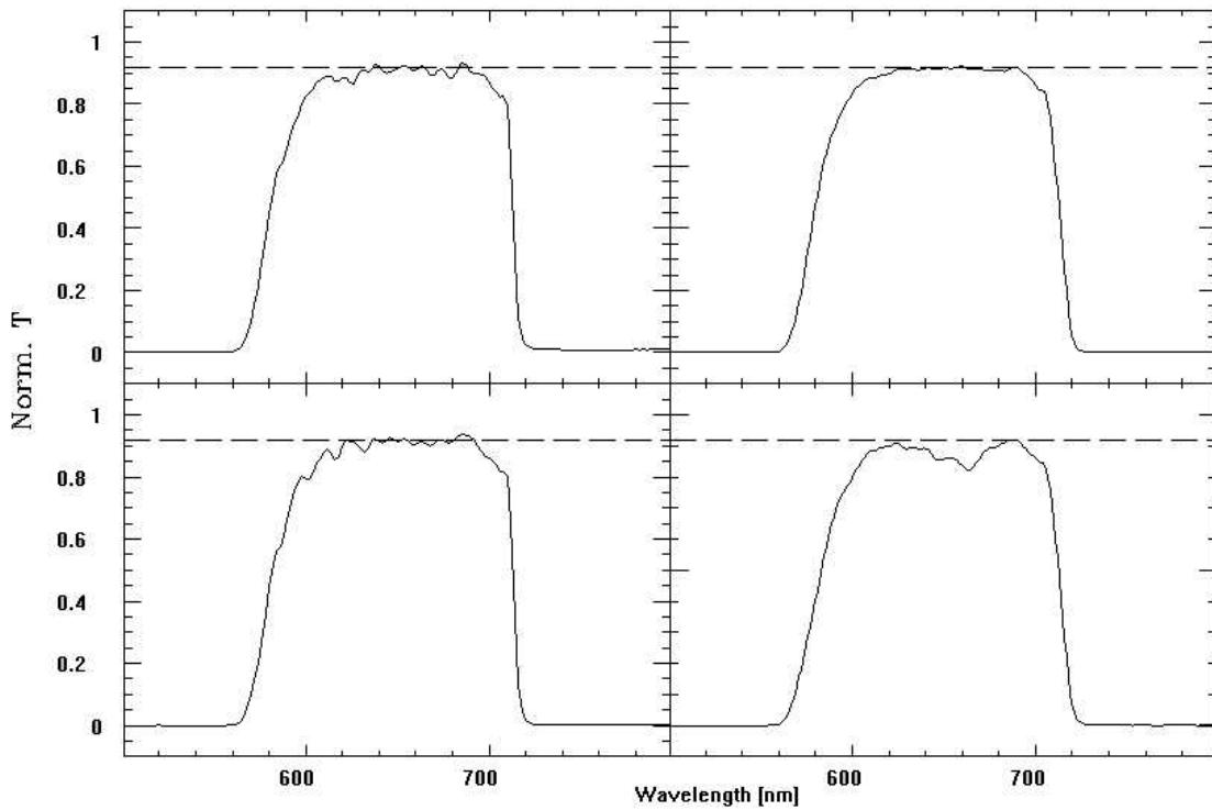
**Figure 22:** R band filter transmission curves
