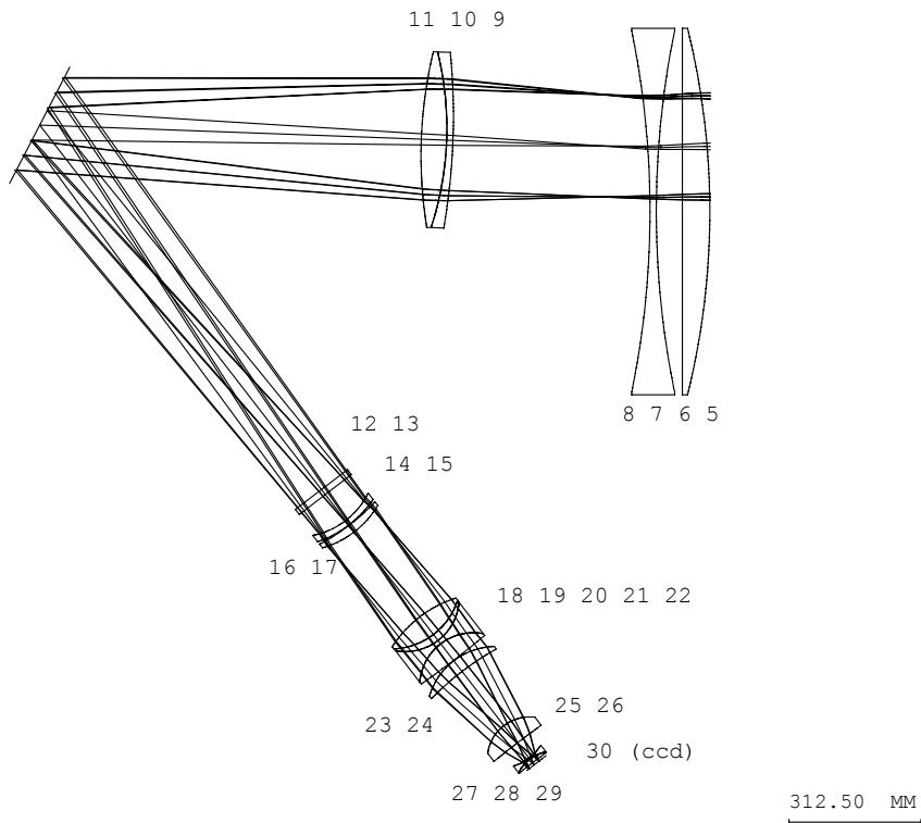
**Figure 3:** VIMOS optical layout (one channel only)
