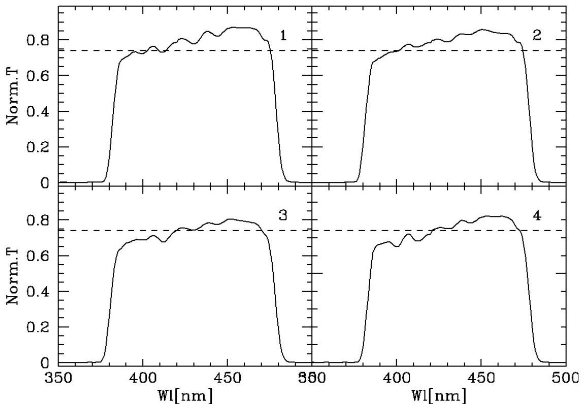
**Figure 20:** B band filter transmission curves
