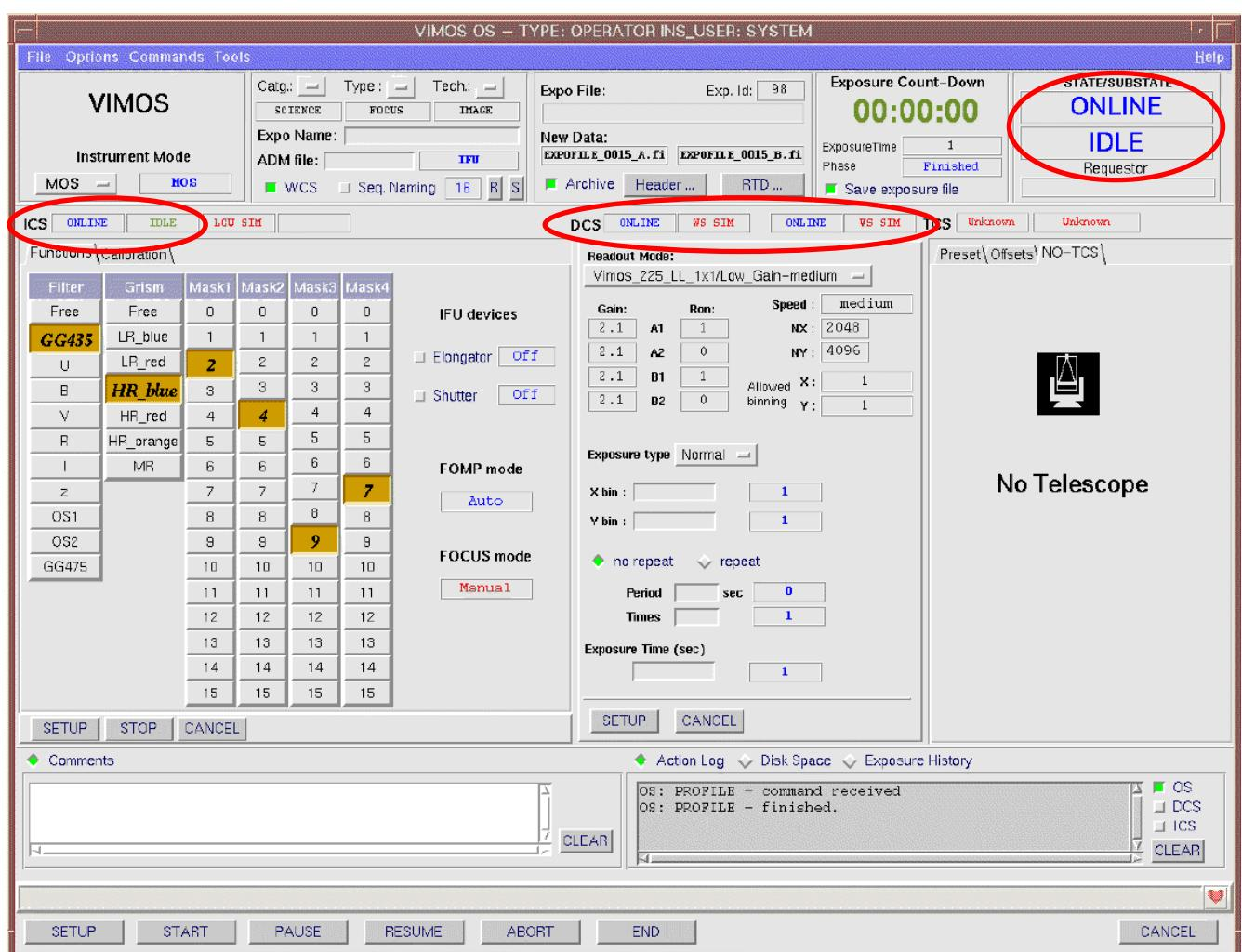
**Figure A.1:** OS panel. At completion of the vmmsStart procedure, the instrument status should be "ONLINE/IDLE" (upper right), as well as the ICS and the 2 DCS environments (left and middle).
