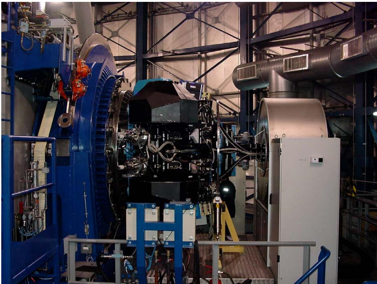
**Figure 6:** The VIMOS instrument installed on the Nasmyth plateform of UT3-Melipal
