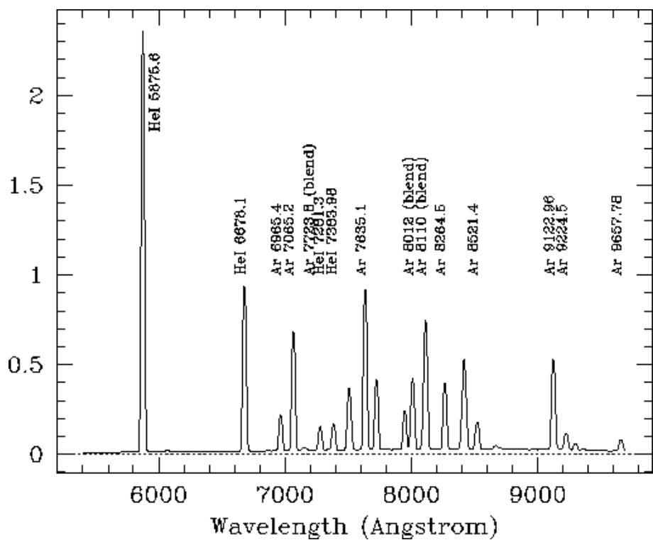
**Figure 31:** He + Ar arc spectrum with the LRRed grism
