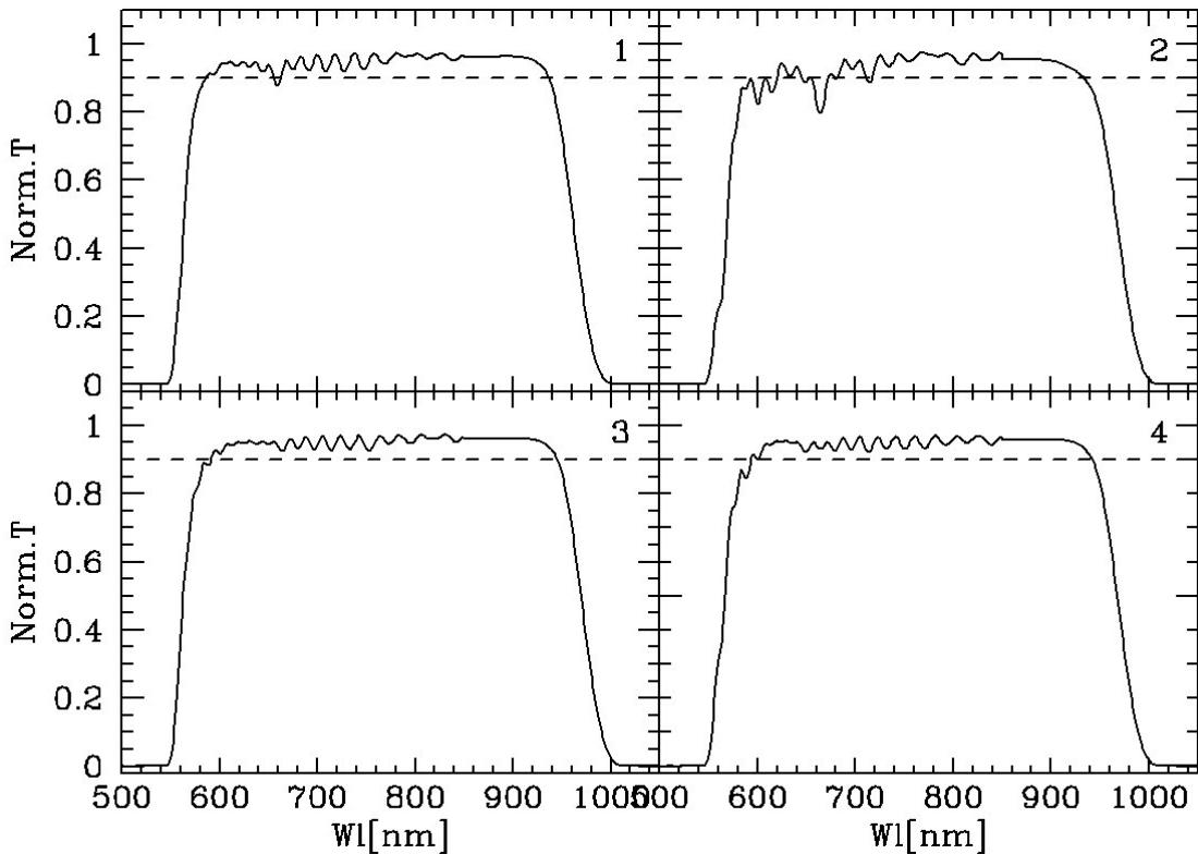
**Figure 26:** OS2 filter transmission curves
