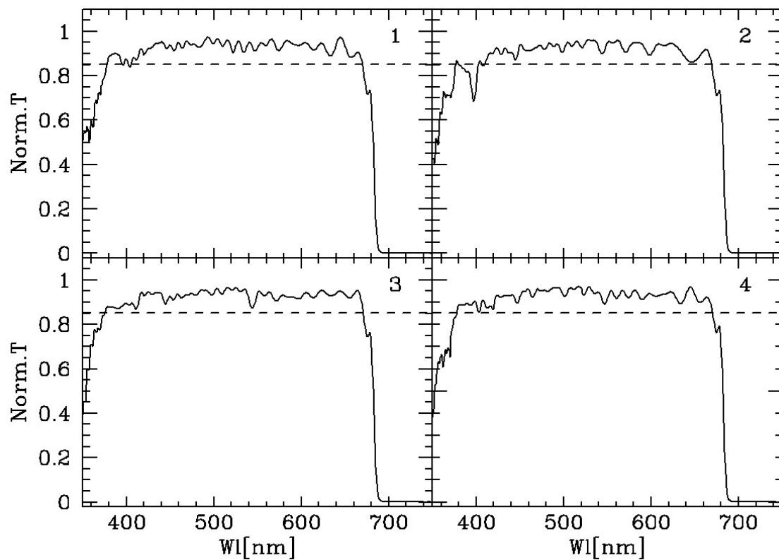
**Figure 25:** OS1 filter transmission curves
