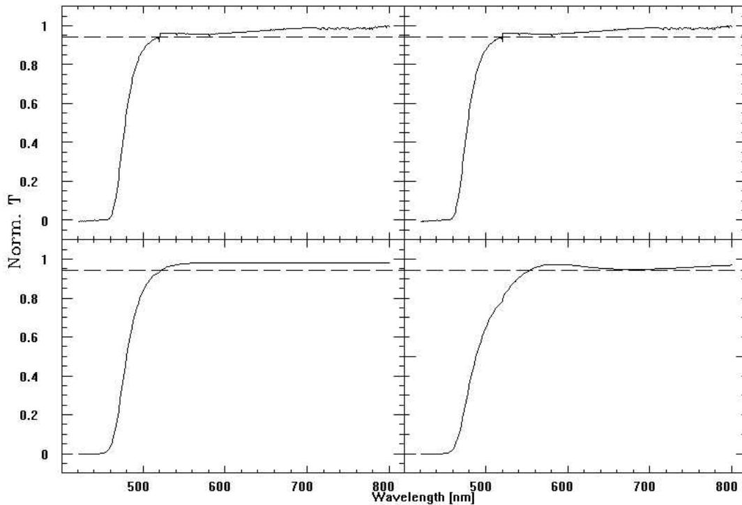
**Figure 28:** GG475 filter transmission curves
