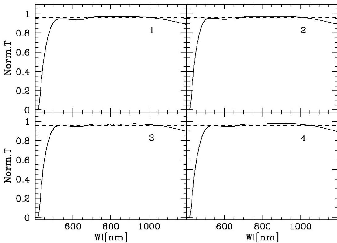
**Figure 27:** GG435 filter transmission curves
