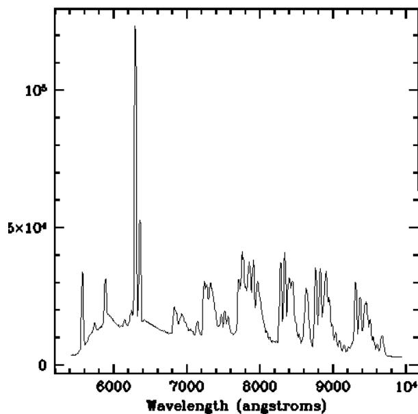
**Figure 29:** sky spectrum, in CCD counts, 1440 sec integration, 1 arcsec slit, LRRED grism
