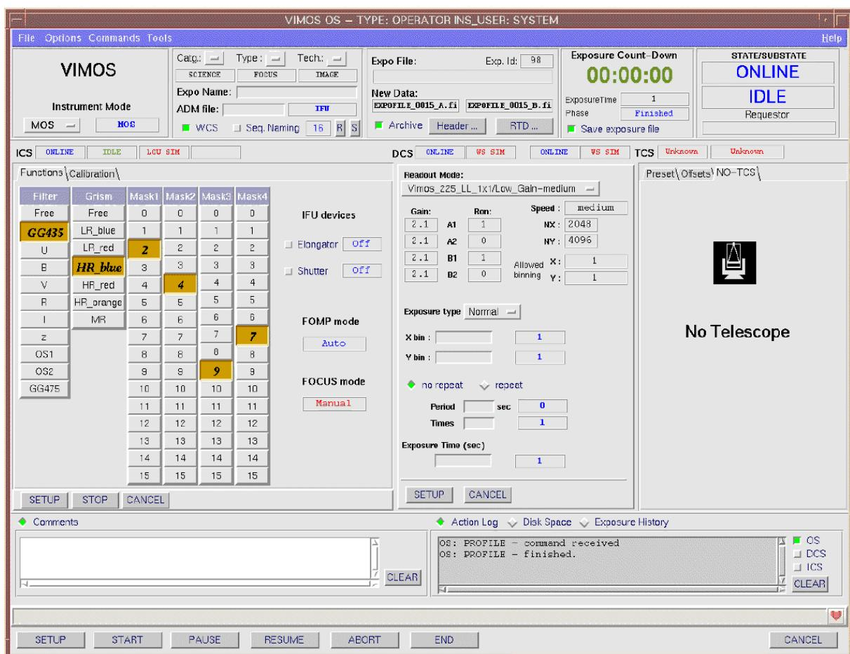
**Figure 7:** VIMOS OS graphical user interface. Left: instrument control panel, Middle, detector control panel. Right: telescope control panel
