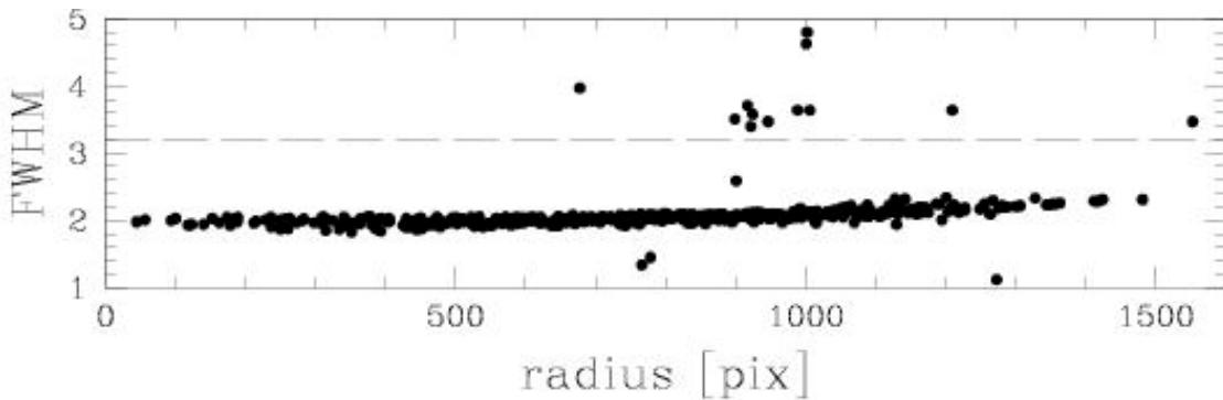
**Figure 9:** Image quality FWHM vs. distance from the optical center, in pixels (quadrant 4). The FWHM measures the images of pinholes 300 microns in diameter distributed in a grid at the mask focal plane. The specification is shown as a dashed line, as FWHM=3.2pix, the measured image quality is ~2 pixels FWHM over the field.
