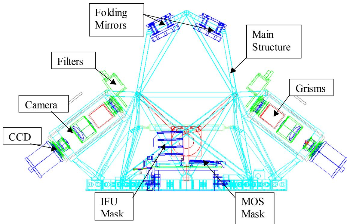
**Figure 4:** VIMOS opto-mechanical layout, top view
