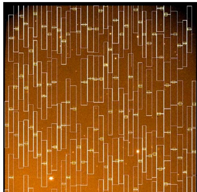
Figure 16: Display of slits selected by vmmmps / SPOC with objects location and spectra extent
