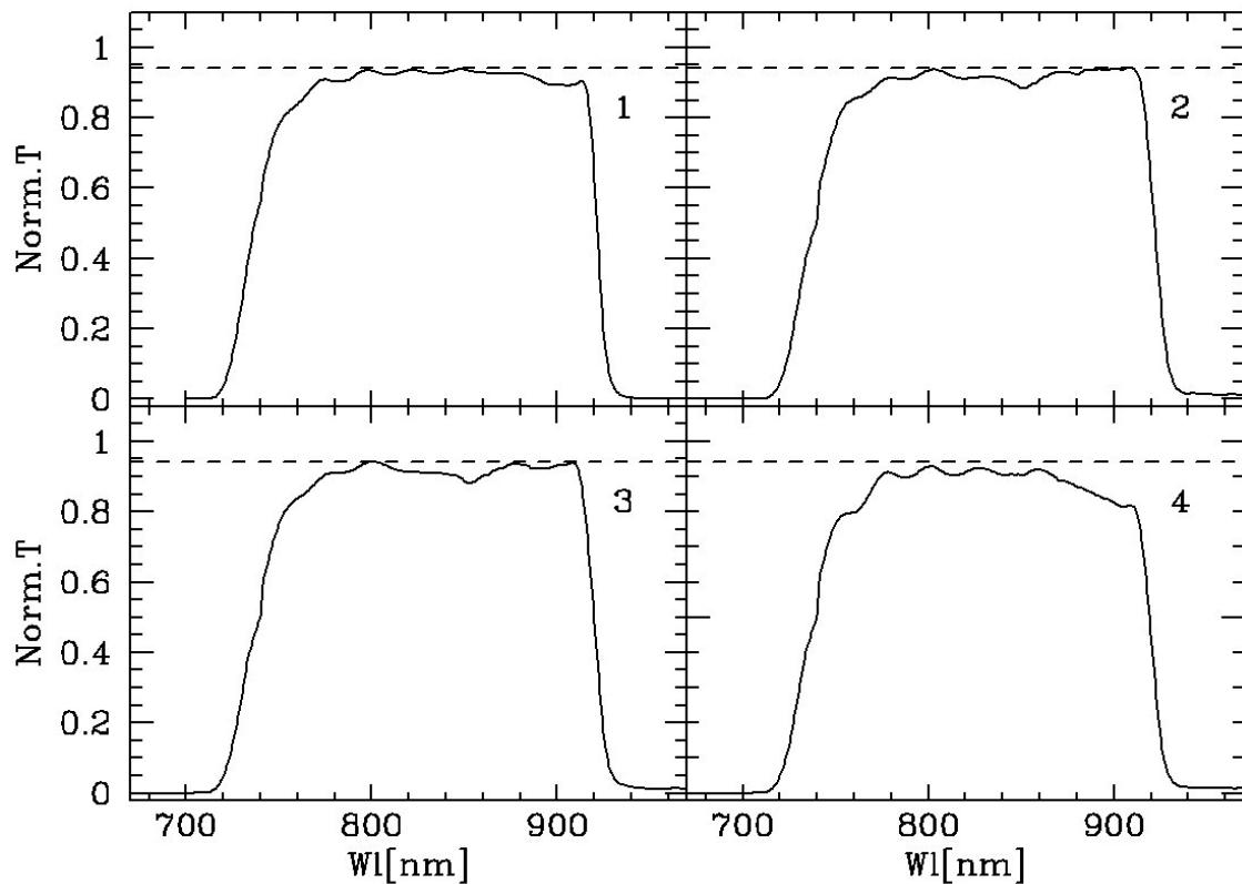
**Figure 23:** I band filter transmission curves
