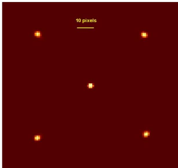
**Figure 10:** PSF variation accross the VIMOS field at the field center and field edges (images of 300 microns holes)
