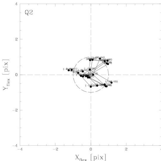
**Figure 11:** flexures measured for channel 2. The circle represents a motion of 1 pixel from central reference.
